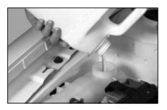
3. Then fill the coolant surge tank with the proper mixture, to the FULL COLD mark.
